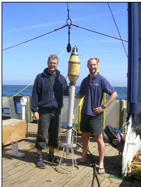
The FLY turbulent dissipation profiler, flanked by Tom Rippeth (left) and Phil Wiles (right).
