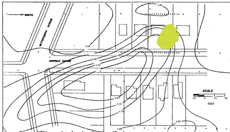
Figure 1.39 Complete Bouguer gravity anomaly map over a near-surface solution cavity in Grand Rapids, MI. Contour interval is 0.05 mGal. The colored area at the northwest end of the gravity anomaly minimum marks the limits of a surface collapse zone. Adapted from Oray and Sanderson (1967).
