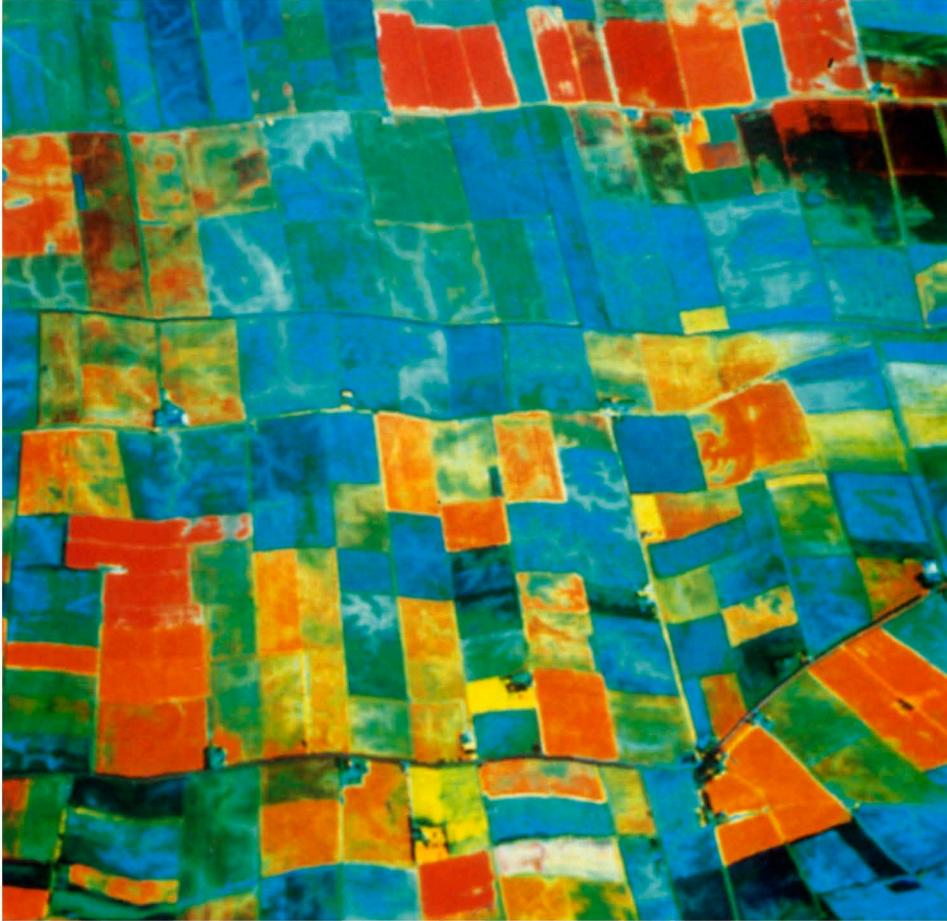
Plate II A false-colour composite image (acquired during the NERC 1986 Airborne MSS campaign) of a part (~5 x 5 km) of Morton Fen, Eastern England. The soil marks and crop marks reveal ancient tidal channels, archaeological features and the variation in soil parent material. Due to changes in inland drainage requirements, influenced significantly by any future sea level rise, further soil changes, resulting from oxidation, wind erosion, compaction or waterlogging, can be monitored using these MSS data and used in impact assessment, allowing consideration of factors such as landscape and archaeological value as well as agricultural benefits. This image was produced by Danny Donoghue.
