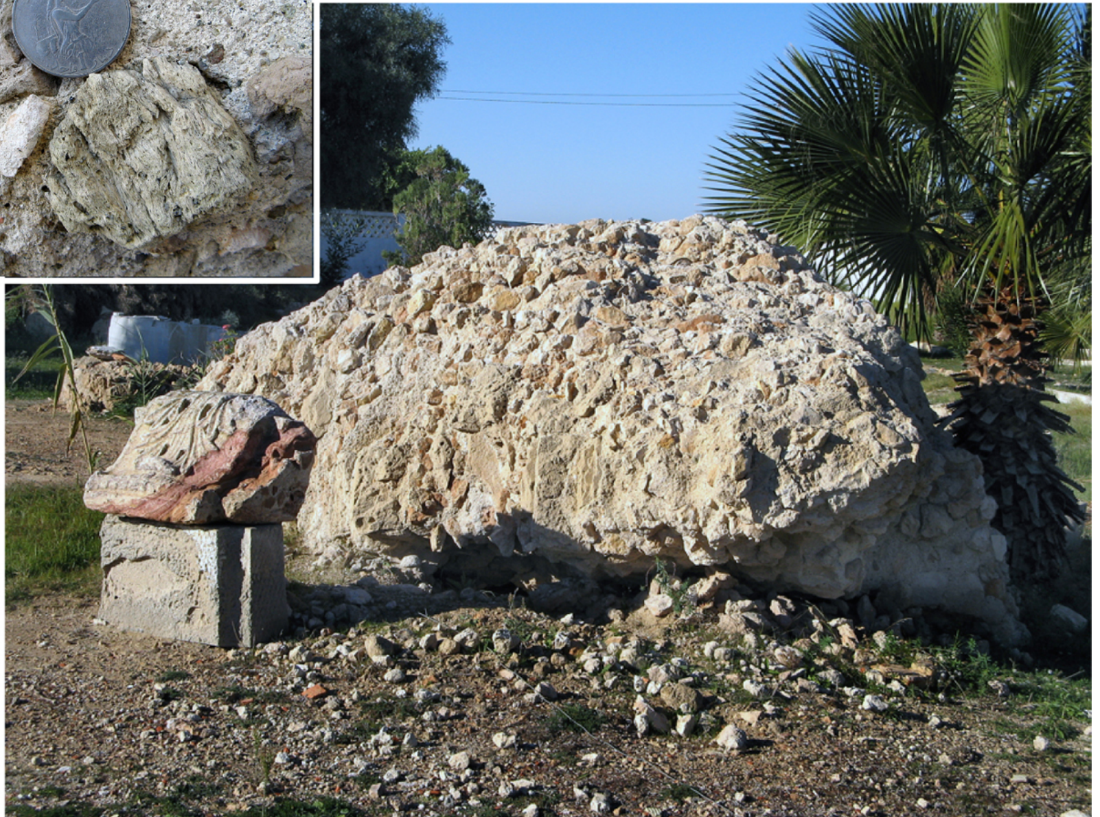
Web Figure 5 (=Figure 10B). East Baths at Leptiminus, Tunisia (late second century CE). Chunk of fallen vaulting with admixture of light colored pumice imported from Pantelleria.
