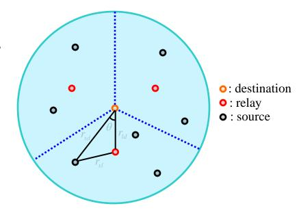
$$r_{sl}(\theta) = \sqrt{r_{sd}^2 + r_{ld}^2 - 2r_{sd}r_{ld}\cos(\theta)}$$
