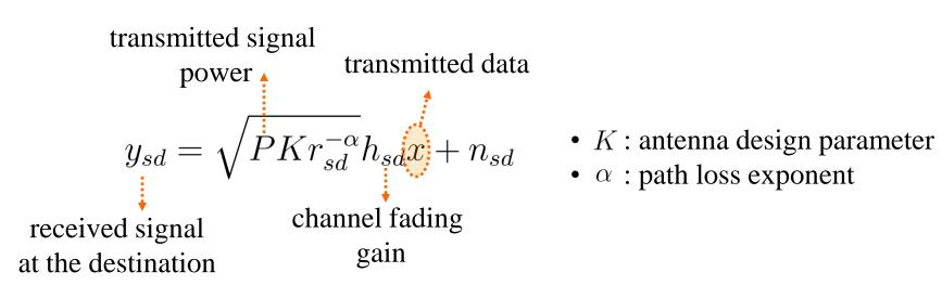
$$SNR(r_{sd}) = \frac{|h_{sd}|^2 K r_{sd}^{-\alpha} P}{N_o}$$
