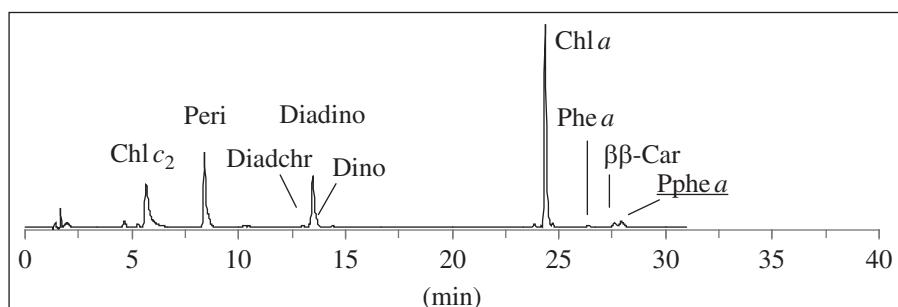
**HPLC chromatogram of a sediment trap sample (system 3)**
