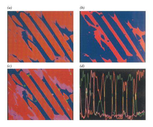
2. Multicolour images of same specimen as in plate 1: (a) 'binary' image of Mg showing areas where Mg X-ray intensity is below (blue) or above (red) threshold; (b) ditto for Al; (c) multiple image showing areas high in Mg (red), Al (blue), Ca (pink), Fe (green); (d) line scan profiles showing distributions of Mg (green), Al (red), and Ca (pink) across centre of scanned area.
