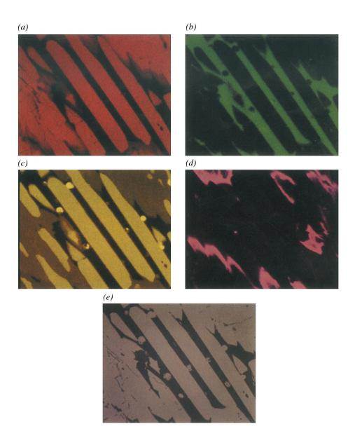
1. Images of microstructure in meteorite: monochrome elemental X-ray images of (a) Mg, (b) Al, (c) Fe, (d) Ca, and backscattered electron image (e) with enhanced contrast to emphasise atomic number differences.
