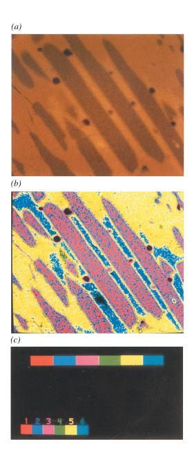
3. Images of Si distribution in same specimen as in plate 1: (a) monochrome, (b) false colours using colour scale shown in (c).
