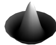
Figure. 6.3: Modal analysis – the first six modes. Silicon plate with radius L = 200 \mu\text{m} and height h = 1 \mu\text{m} . The plate is discretized with N_1 = 20 degrees of freedom in the r -direction and N_2 = 20 degrees of freedom in the \theta -direction (total of 400 DOF!). Note that modes n = 2 and n = 3 are degenerate modes (also modes n = 4 and n = 5 ). Due to symmetry in the \theta -direction, there are infinite mode shapes that correspond to these modes – we can imagine any arbitrary rotation of these two as a valid mode shapes.
