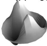
Figure. 6.3: Modal analysis – the first six modes. Silicon plate with radius L = 200 \mu\text{m} and height h = 1 \mu\text{m} . The plate is discretized with N_1 = 20 degrees of freedom in the r -direction and N_2 = 20 degrees of freedom in the \theta -direction (total of 400 DOF!). Note that modes n = 2 and n = 3 are degenerate modes (also modes n = 4 and n = 5 ). Due to symmetry in the \theta -direction, there are infinite mode shapes that correspond to these modes – we can imagine any arbitrary rotation of these two as a valid mode shapes.
