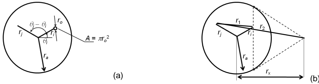
Figure. 6.1: A sketch of the plate introduces the geometric parameters r_i , r_j , r_1 , r_2 , r_x , and r_a used in Eqs. (6.1)-(6.4).
