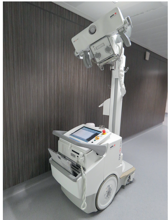
Figure 2.12 Mobile radiographic system for bedside imaging (DX-D 100, Agfa Healthcare). It uses a wireless portable detector with needle-shaped cesium iodide (CsI) scintillator and active matrix array.
