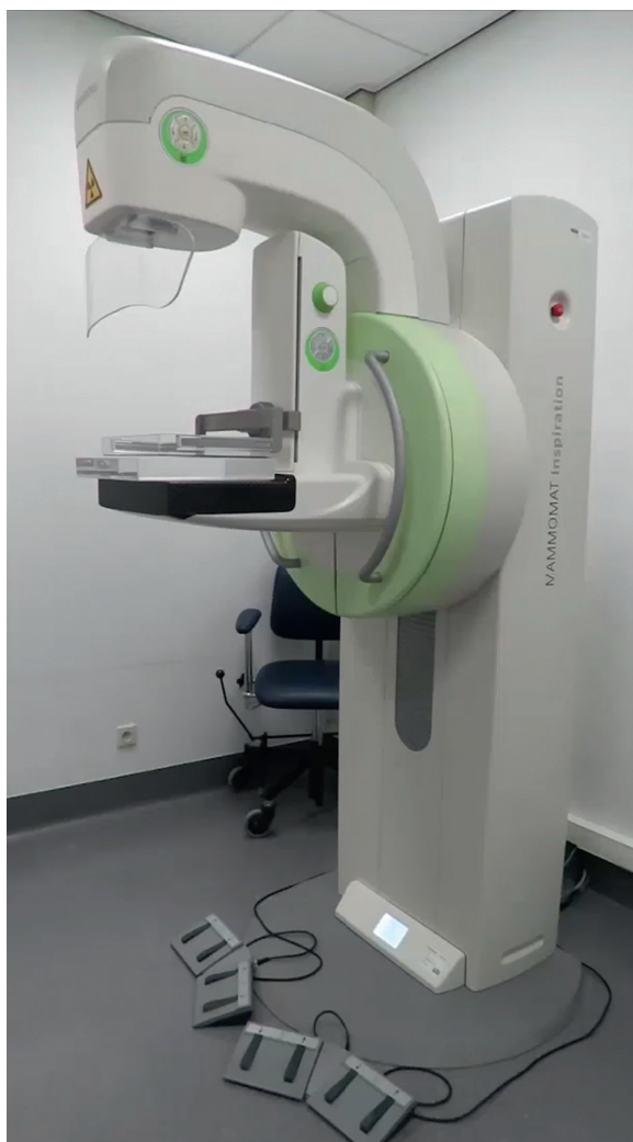
Figure 2.13 Digital mammography system employing direct X-ray conversion with amorphous selenium (Mammomat Inspiration, Siemens Healthcare). This system can also be used for digital tomosynthesis by rotating the X-ray tube from left to right (see Section 3.7.1).
