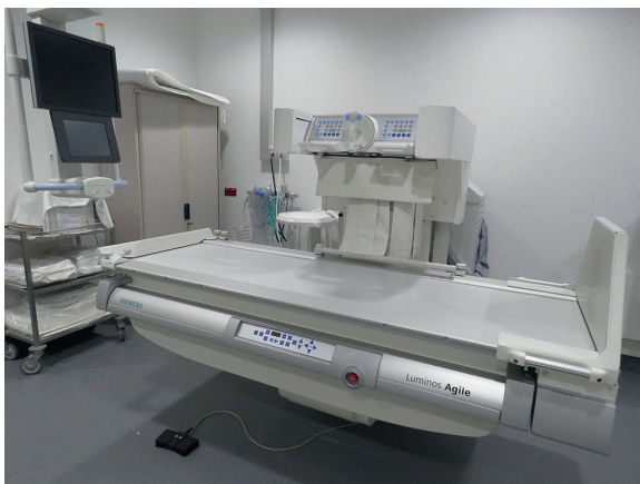
Figure 2.11 Similar system as Figure 2.10(a) but the X-ray tube is placed under the table and an easily movable detector with radiation protective shield above the table, suitable for patient-side examinations (Luminos Agile, Siemens Healthcare).
