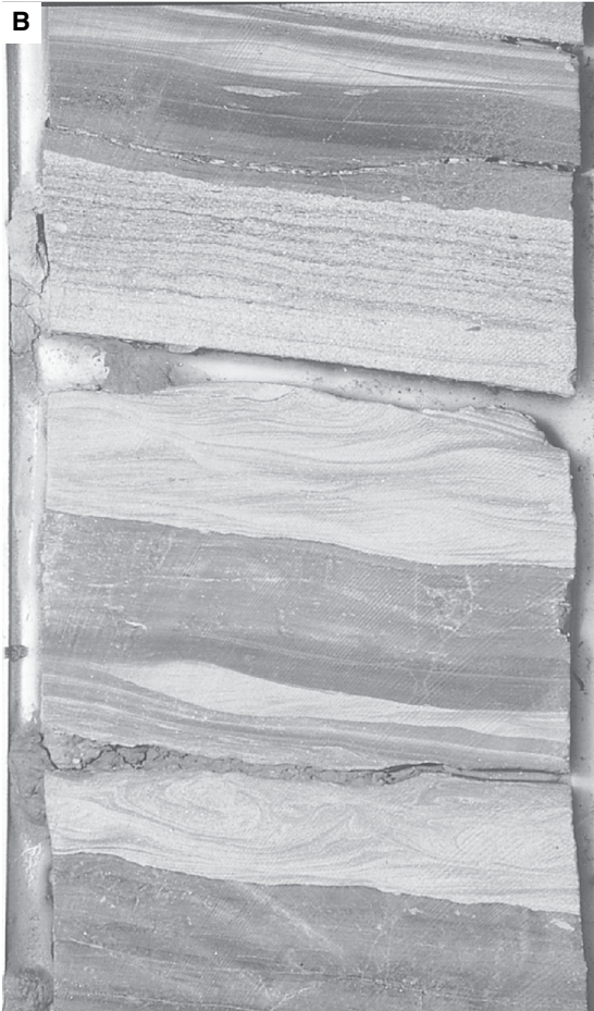
FIGURE 18.25 (A) Interpreted overbank deposits from Marnoso-arenacea, Italy, showing a thickening-upward sequence. (B) Interpreted muddy levee deposits in a 10-cm-wide core from the Lange Formation, offshore Norway. The light-colored sandstone beds contain climbing-ripple cross strata and convolute lamination. (C) Tabular, sheet-like turbidites with thickening- and thinning-upward sequences, Lower Ross Formation, western Ireland. Pictures Courtesy of Henry Posamentier.
