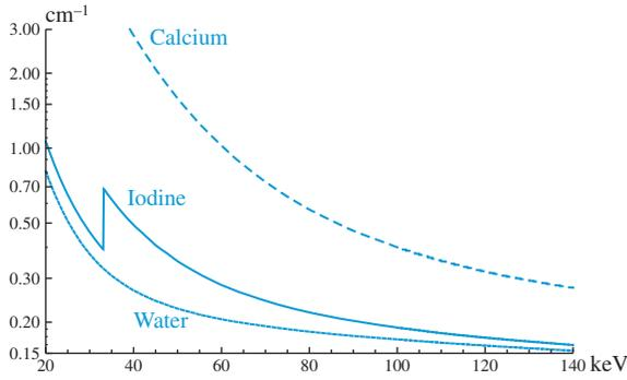
**Figure 3.22** Linear attenuation coefficient as a function of the energy for calcium (Ca), water, and the contrast agent iodine (I) in water (10 mg/ml). Note the K-edge discontinuity of I at 33.2 keV.
