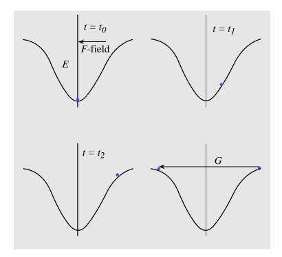
The motion of an electron in a band in the absence of any scattering and in the presence of an electric field. The electron oscillates in *k*-space gaining and losing energy from the field.
