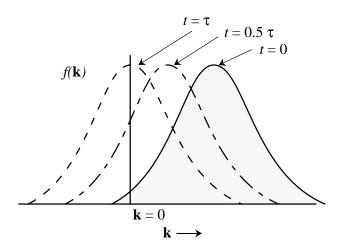
This figure shows that at time t = 0, the distribution function is distorted by some external means. If the external force is removed, the electrons recover to the equilibrium distribution by collisions.
