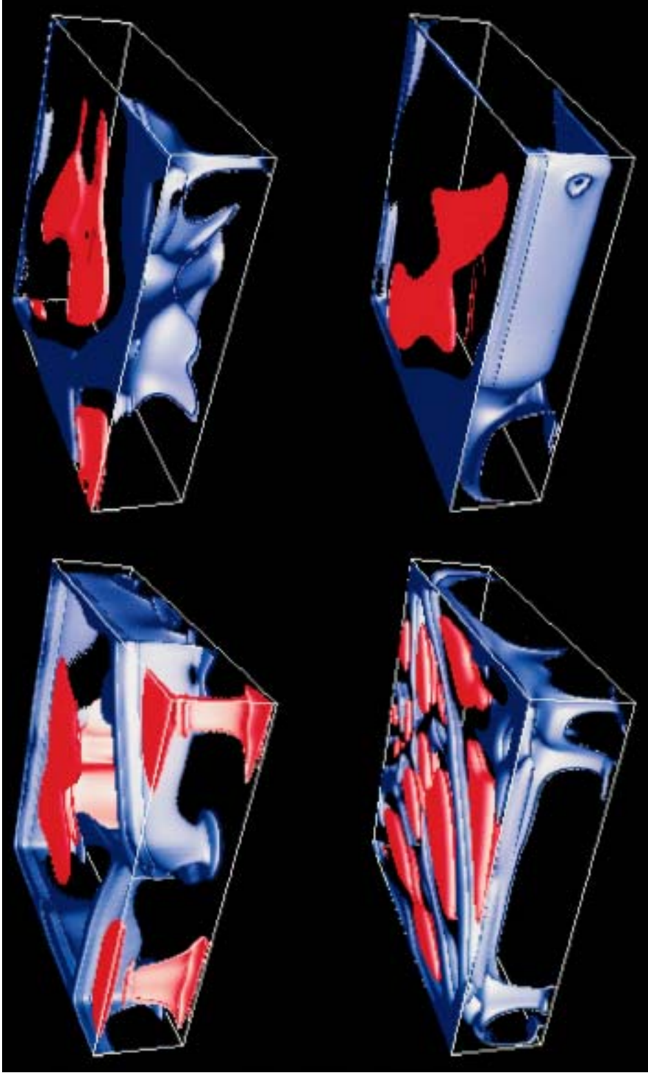
Figure 14.19. Cold downwellings (blue) and hot upwellings (red) for the three variable viscosity phase change cases. Plotted are isosurfaces of residual temperature, i.e., temperature relative to the horizontally averaged temperature profile, showing where the temperature is \pm 0.1 from the horizontal average. (a) (Top left) constant viscosity case 1, (b) (lower left) variable viscosity case 2, (c) and (d) (right) variable viscosity with a yield stress (case 3) at two different times.
