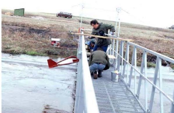
**Figure A-1.** Helley-Smith bedload sampler deployed from a measuring bridge.
