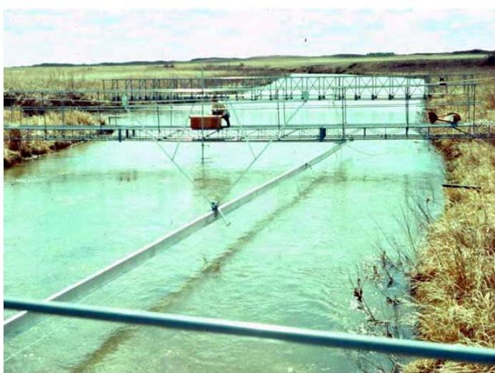
*Figure A-3. Operation of a high-resolution depth profiler from moveable railways attached to bridges over a small river*
