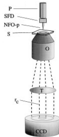
Fig. 10.27. Apparatus for launching SPs on a metallic film by a near field tapered fiber probe and observing the propagating SPs. Reprinted with permission from B. Hecht, H. Bielefeldt, L. Novotny, Y. Inouye, and D. W. Pohl, Phys. Rev. Lett. 77 1889 (1996). © 1996 by the American Physical Society. [24]
