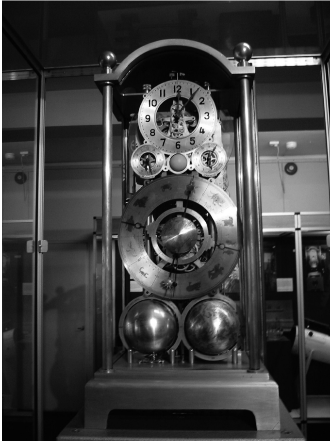
Astronomical clock (number 3) designed and made in Norway by Rasmus Sørnes. Finished in 1954, it computes a large number of time/astronomical values including sidereal time, sunsets and sunrises, Gregorian date, solar and lunar eclipses, precession, tides, the positions of the planets, and many other things. (Courtesy of the Borgarsyssel Museum, Sarpsborg, Norway.)
