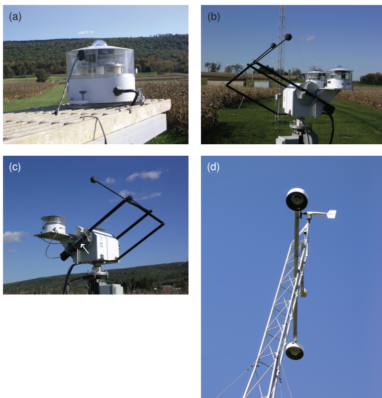
Figure 6.1 Radiation instruments at the Penn State, Pennsylvania SURFRAD Network site: (a) pyranometer used to measure incoming shortwave radiation on a horizontal surface, (b) a continuously shaded pyranometer (near) and pyrgeometer (far) used to measure incoming diffuse shortwave and incoming longwave radiation, respectively, (c) tubular pyrhelometer (see arrow) mounted on a solar tracker to measure direct-beam solar radiation at normal incidence, and (d) inverted pyranometer and pyrgeometer on tower to measure reflected shortwave and outgoing longwave radiation from the ground surface (photographs by D. DeWalle).
