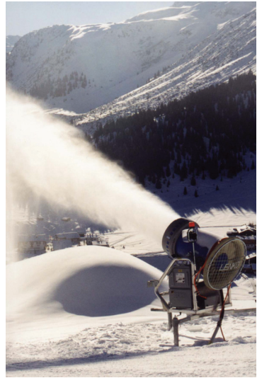
Figure 12.11 Ratnik low-energy modified snow gun (left) and modified fan-type Lenko snow gun (right) being used to augment snowpack for skiing (courtesy of Ratnik Industries, Inc. and Lenko Quality Snow, Inc., respectively).
