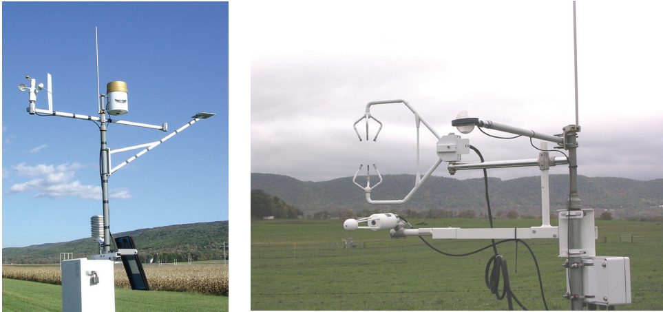
Figure 6.5 Solar-powered climate stations equipped with data loggers (left) are used to provide data (wind speed, air temperature, humidity) to support computations of snowpack convective exchange. The addition to climate stations of sonic anemometers (top right), fine-wire thermocouples, and high-speed open-path gas analyzers for CO 2 and water vapor (bottom right) allows computation of convective exchange using the eddy covariance method (photographs by D. DeWalle).
