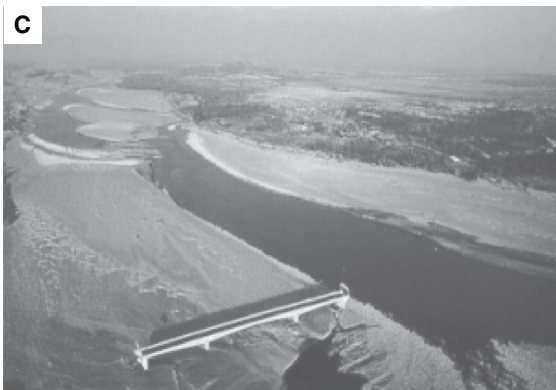
FIGURE 13.33. Bank erosion and human activities. (A) Failed riprap and serious bank erosion along a creek in New York State. Remains of concrete riprap and bridge piers lie in the river. (B) Bank erosion undercutting a railway line in northwest Argentina. (C) River and roads moved during a flood in central America, but this bridge did not. (D) Bank protection on an Alpine river, Switzerland. Images (E) and (F) show riprap along the Brahmaputra River, Bangladesh (photos courtesy of Jim Best). Modified from Bridge (2003).
