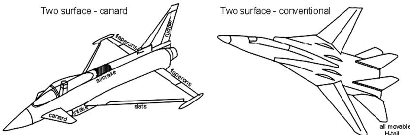
Figure 12.16 Typical modern fighter aircraft
