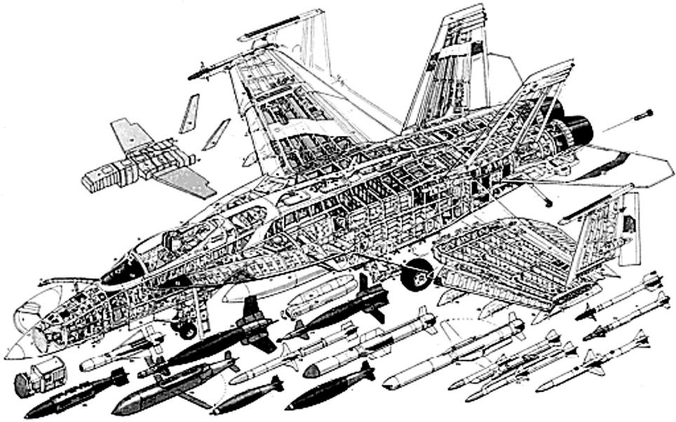
Figure 6.17. USAF F18 details showing internal structural layout and armament load
