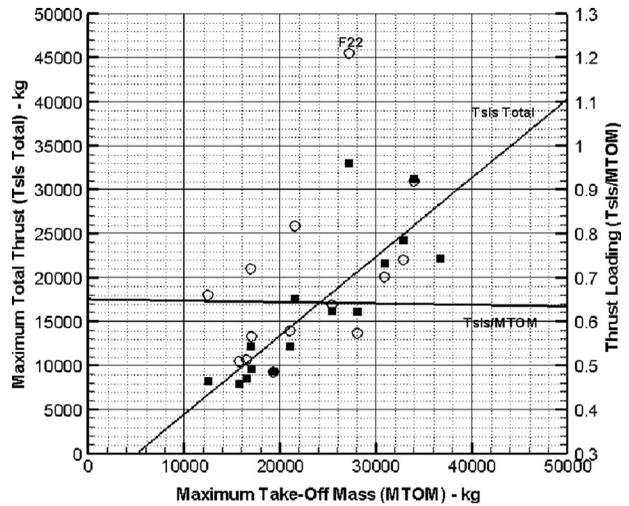
Figure 4.36. Aircraft weight versus total take-off thrust
