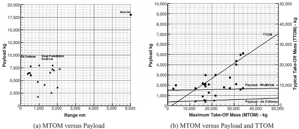
Figure 4.32. Military aircraft payload – range (no drop tank or refueling)
