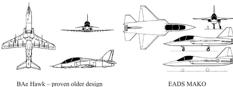
Figure 4.38. Advanced jet trainer aircraft capable of close support combat
