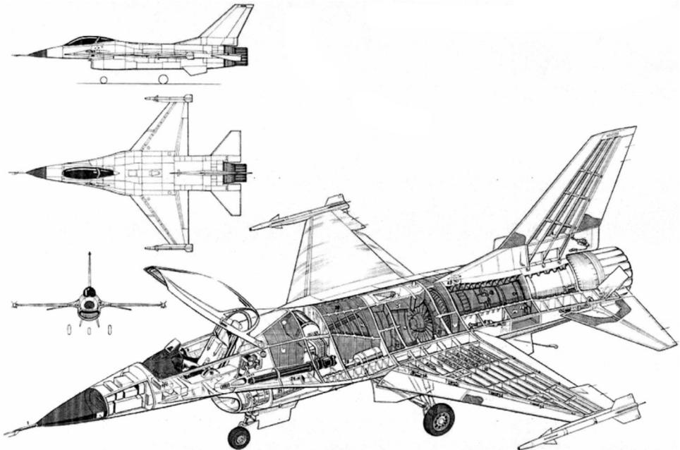
Figure 2.5 A diagram of the General Dynamics (now Boeing) F16 – internal layout
