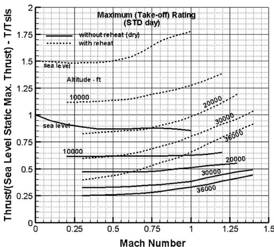
Figure 10.51. Military turbofan engine with and without reheat ( $BPR = 0.75$ ). Take 90% of maximum rating as the maximum continuous rating
