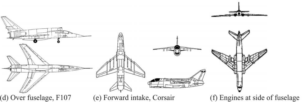
Figure 4.41. Options for engine positions of some older designs
