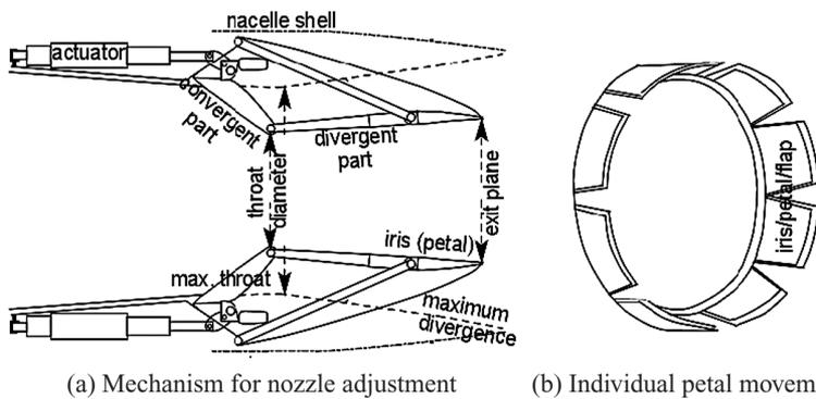
Figure 10.28. Military aircraft nozzle adjustment scheme (from Ref [10.19])
