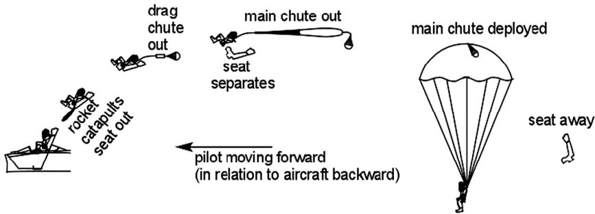
Figure 15.44. Typical ejection sequence showing separation of seat and parachute deployment
