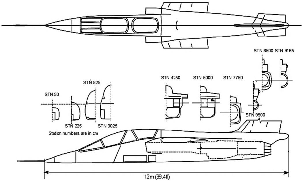
Figure 6.20. AJT fuselage layout
