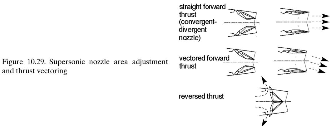
Figure 10.29. Supersonic nozzle area adjustment and thrust vectoring
