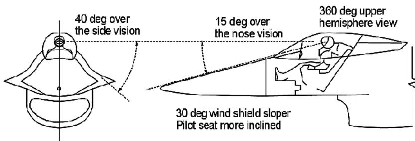
Figure 6.16. Flight deck (cockpit) layout – military aircraft
