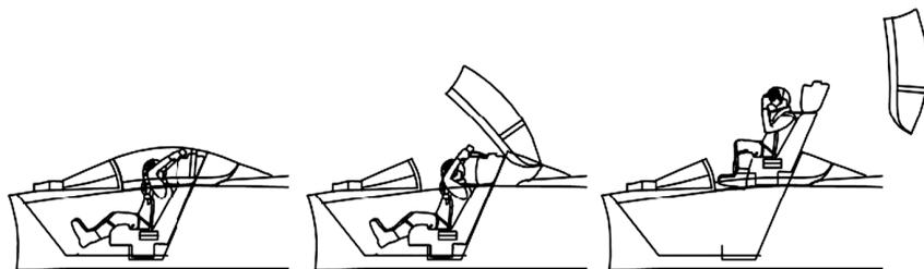
Figure 15.43. Typical ejection sequence
