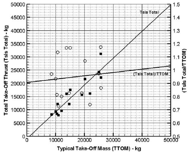
(total  $T_{SLS}/MTOM$ ) is averaged around 0.65 but (total  $T_{SLS}/TTOM$ ) exceeds 1. Later generations of combat aircraft have pushed the thrust-to-weight ratio to more than one that would permit aircraft to accelerate in vertical climb. The F22 has the highest thrust loading, as well as the lowest wing loading.
