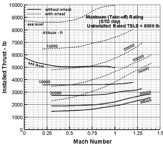
Figure 13.4 Installed maximum rating – military turbofan ( $BPR = 0.75$ )
