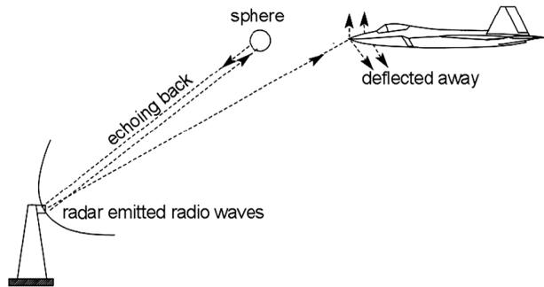
RCS area is defined as the projected area of an equivalent perfect reflector with uniform properties in all directions, such as from a sphere, and which returns the same amount of power per unit solid angle in steradians as the object under consideration.
