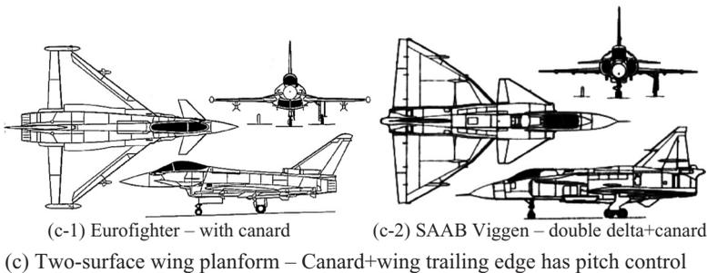
Figure 4.37. Fighter aircraft configurations
