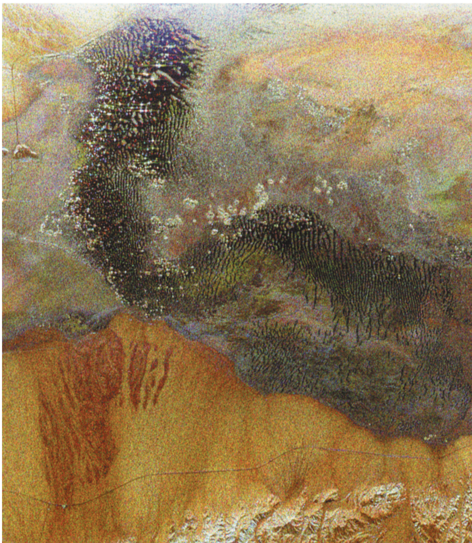
Figure 7.16. AIRSAR three-wavelength (red = 5.7 cm, green = 24 cm, blu = 68 cm wavelength) HH-polarization image of sand dune field (top center) in Death Valley, CA. Image width 8 km. Note the bright glints from radar-facing dune slopes near the top of the image (courtesy NASA/JPL).
