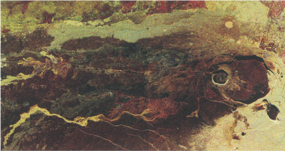
Figure 6.8. Three-wavelength color composite HV-polarization radar image of Kilauea volcano and Ka'u desert, Hawai'i. Red tones correspond to C-band (5.7 cm), green to L-band (24 cm), and blue to P-band (68 cm) echoes. (Calibrated data courtesy T. Farr, JPL, and P. Mouginis-Mark, University of Hawaii).
