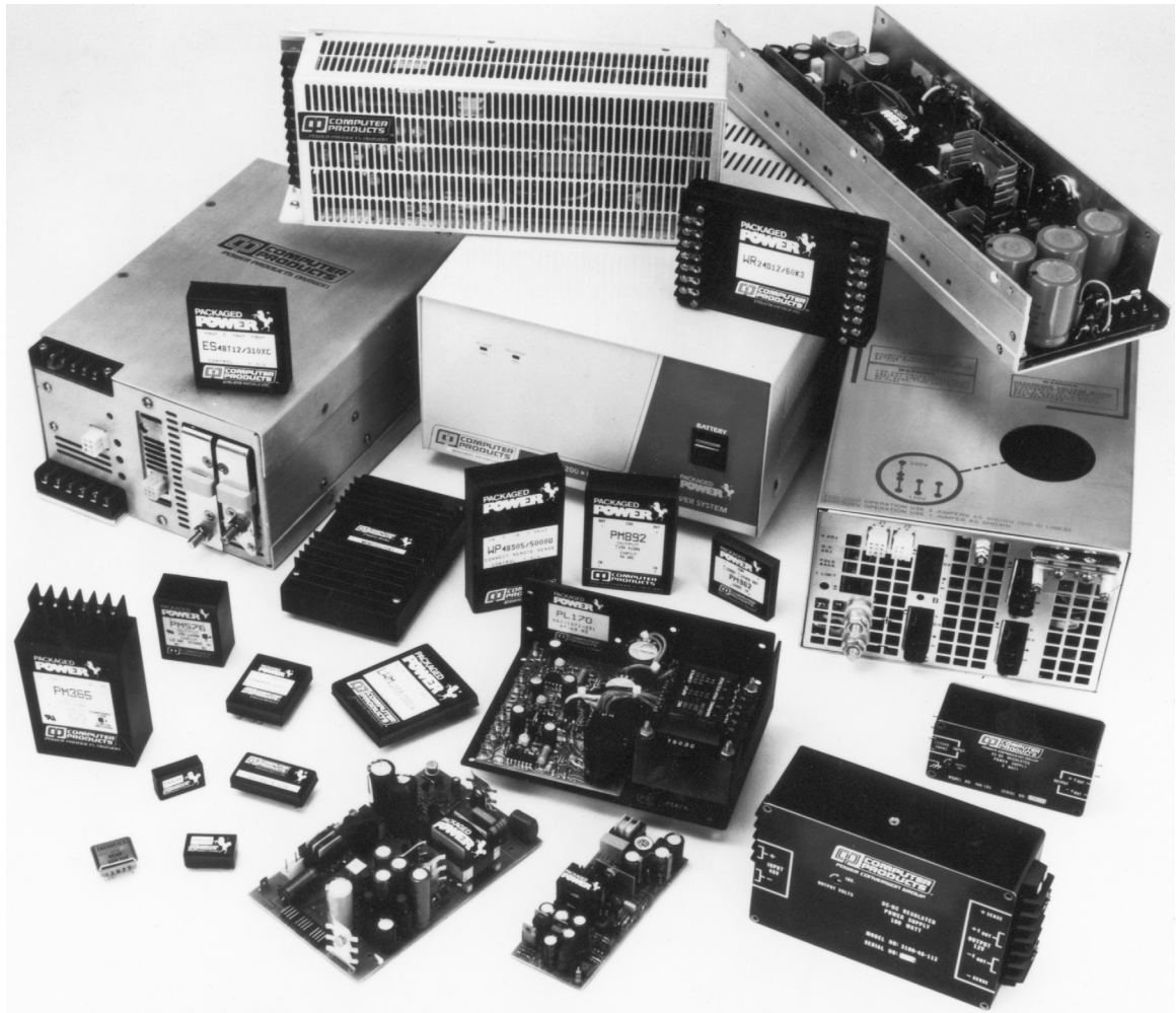
Figure 9.97. Commercial power supplies come in a variety of shapes and sizes, including potted modules, open-frame units, and fully enclosed boxes. (Courtesy of Computer Products, Inc.)
