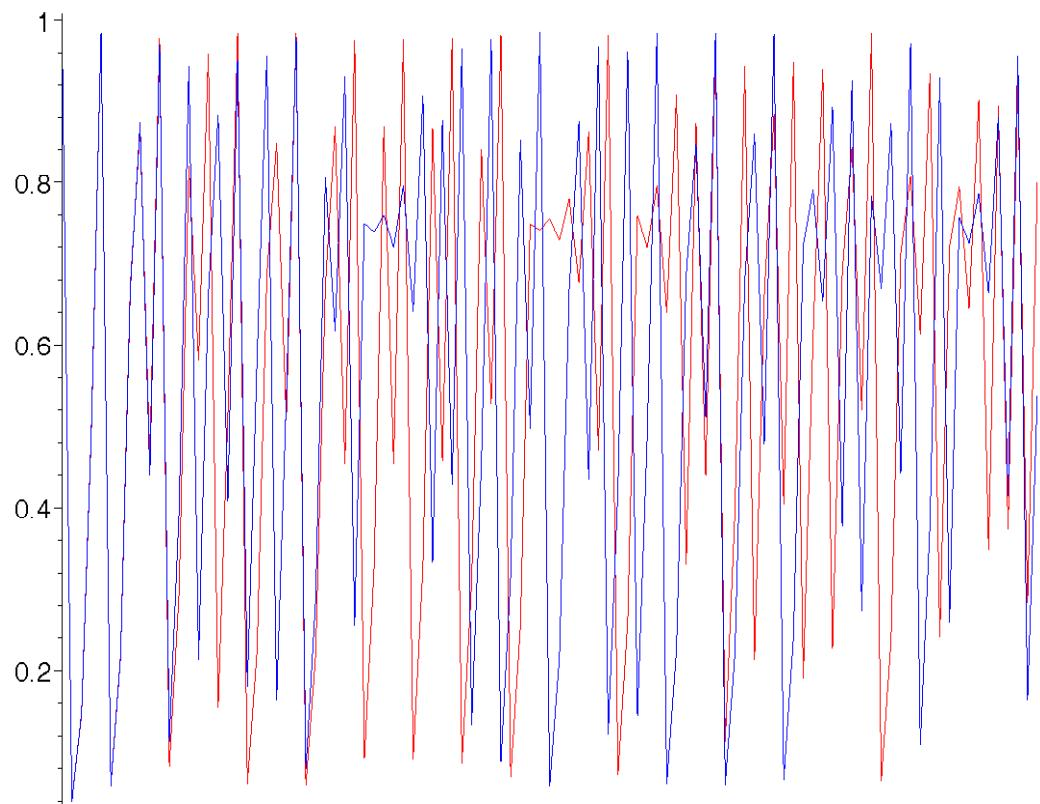
As can be seen from the graph, with just a minor change in the initial condition the two series soon begin to differ.
