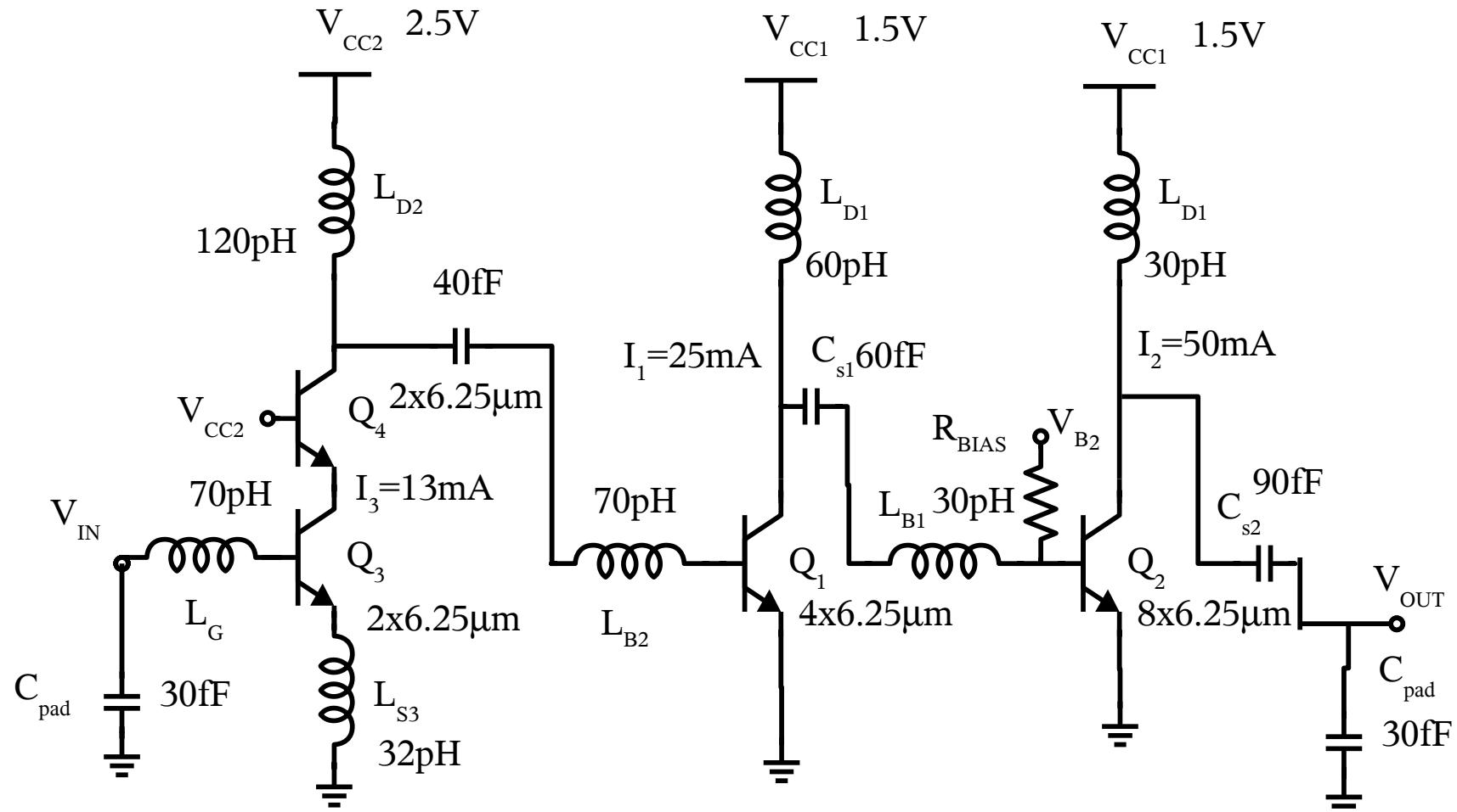
$$P_{sat} \leq \frac{I_{DC} \cdot V_{CC1}}{2} = \frac{44\text{mA} \cdot 1.5\text{V}}{2} = 33\text{mW} = 15.2\text{dBm}$$
