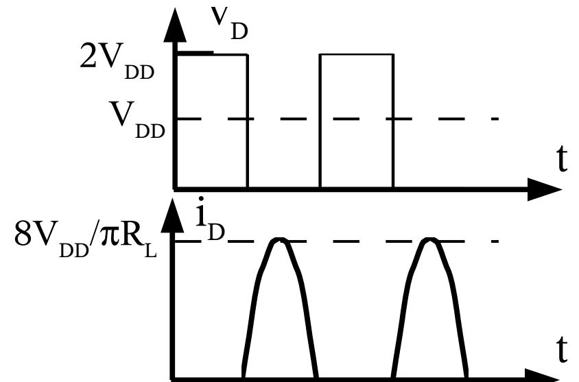
$$Z_L(f_0) = R_L; Z_L(2k \times f_0) = 0; Z_L[(2k+1) \times f_0] = \infty$$
