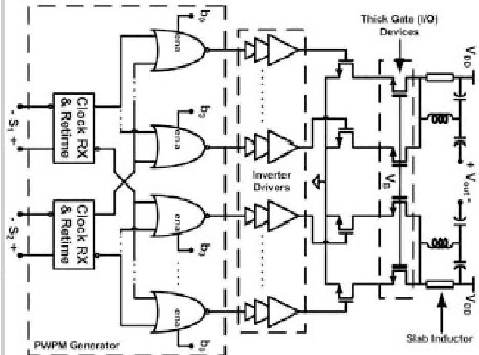
Figure 31.5.2: Schematic of the Class-E PWPM PA.
