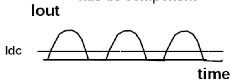
In Class B,  $I_{dc} \sim K I_{max} \sim \sqrt{P_{out}}$
