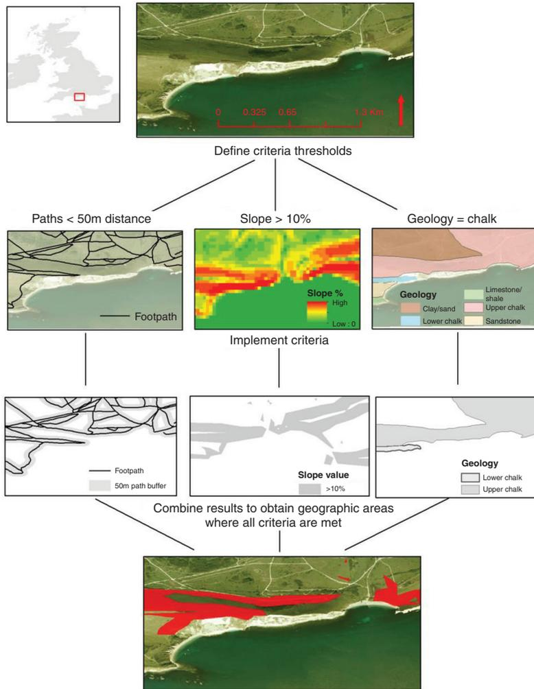
**Figure 2** A hypothetical illustrative example of multi-criteria spatial analysis at Worbarrow Bay near Lulworth Cove along the coastline of southern England. The risk of injury from rock falls can be modelled based on distance to footpath, topographic slope and underlying geological character. Text boxes indicate key parts of the process of multi-criteria analysis.
