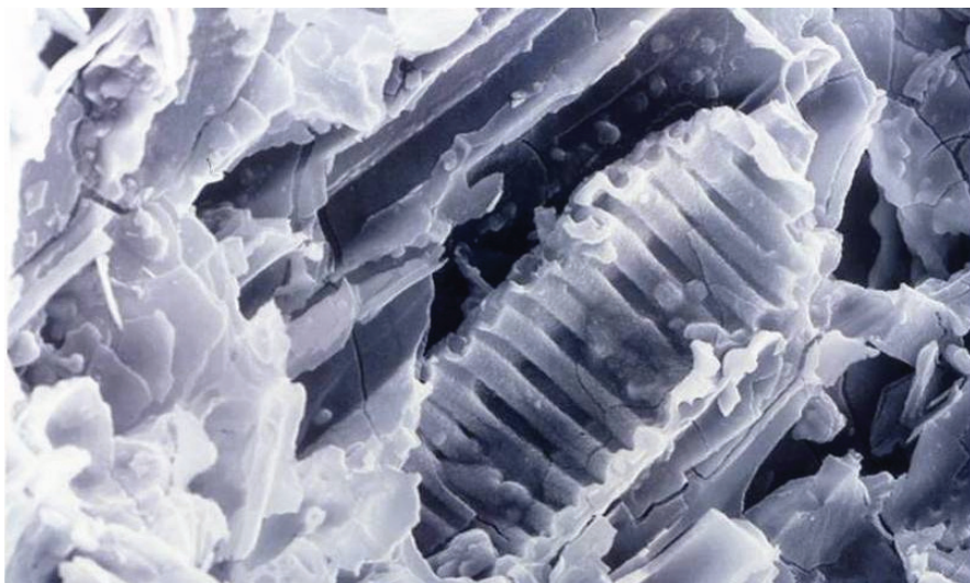
FIGURE 3.14. ESEM scanning electron photomicrograph showing spiral thickening of wood hardwood cells; uncoated, x2100 magnification. From this view it appears that the copper corrosion products are deposited over the thin spiral cellular structures.
