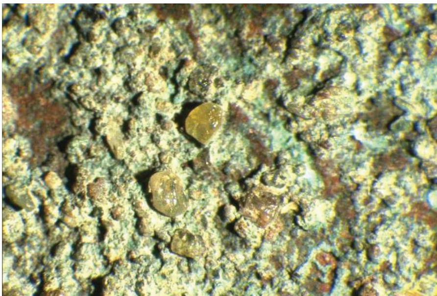
FIGURE 3.2. Another region of Plaque I with concreted soil minerals and small botryoidal growths of malachite overlying the cuprite layer; x40 magnification.
