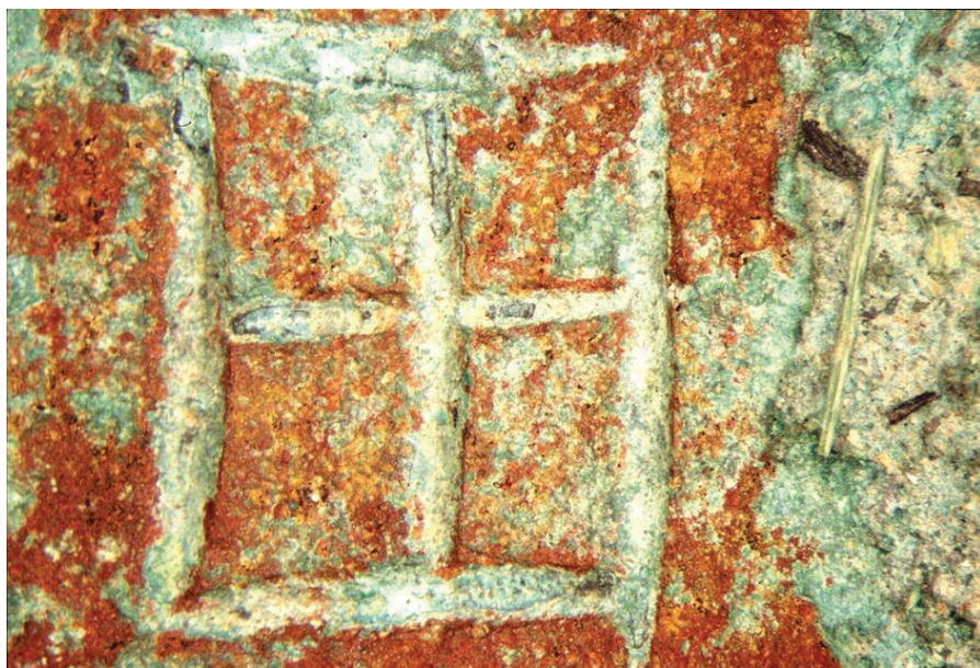
FIGURE 3.1. Photomicrograph of lettering on Plaque I preserved in cuprite; x40 magnification.
