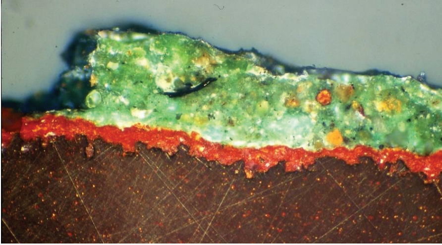
FIGURE 3.8. Unetched cross polar view of the cross section through Plaque I showing well-crystallized cuprite patina under a complex malachite crust. The tiny red spots visible in this section are of cuprite, showing that the copper was smelted from quite pure oxidized ores; x280 magnification.
