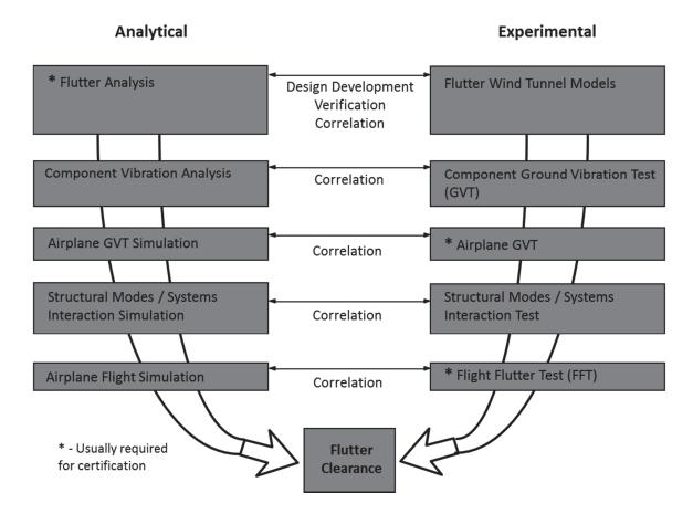
Figure 5.18: Schematic of interaction between analysis and test in certification; from Niedermeyer (2014), Federal Aviation Administration, used with permission
