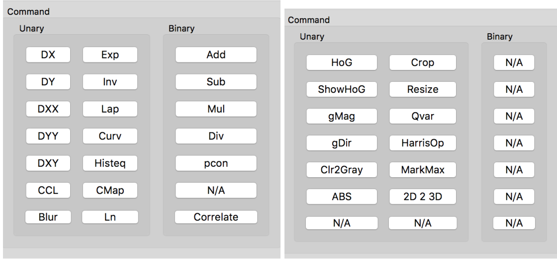
FIGURE 6. (LEFT) Image operations available in mode 0. (RIGHT) Operations available in mode 1. These operations are performed on the eight floating point image buffers.
