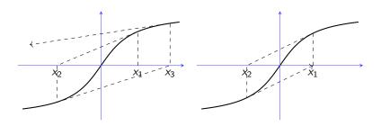
In the first example, the sequence moves away from the solution of f(x) = 0. In the second example, it cycles repeatedly through the same two values.
