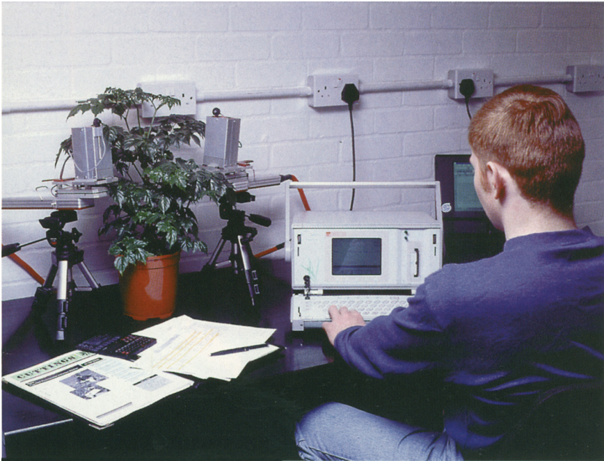
XIII The ADC 2250 for measurements of gas exchanges on the infra-red absorption principle. The high-performance Omega optical bench provides simultaneous absolute and differential gas measurements. (Courtesy: ADC Bioscientific Ltd, Hoddesdon, UK.)
