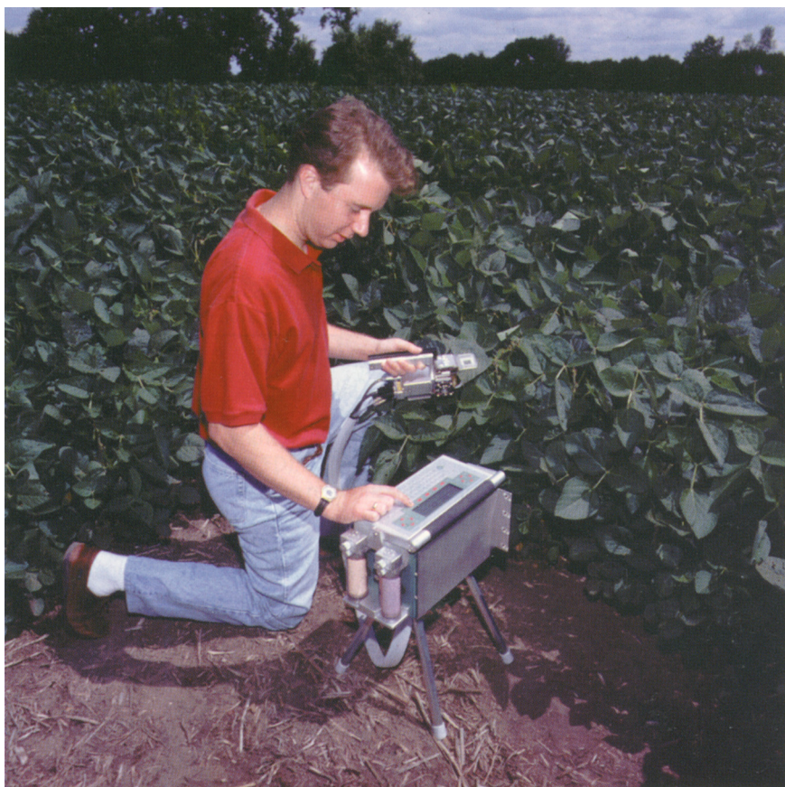
XV The LI-6400 Portable Photosynthesis System for measurement of canopy of \text{CO}_2 gas exchange and instantaneous estimation of light conversion efficiency. (Courtesy: LI-COR Inc., Lincoln, Nebraska, USA.)
