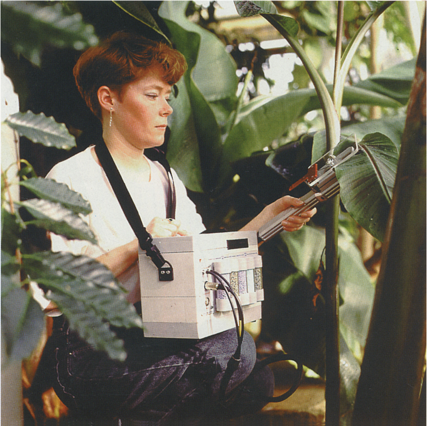
XII Advanced Portable LCA-4 IRGA for photosynthesis and transpiration measurements. (Courtesy: ADC Bioscientific Ltd, Hoddesdon, UK.)
