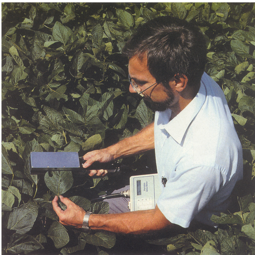
XIV Portable leaf area meter for measurements of areas of leaves in the field and laboratory. (Courtesy: LI-COR Inc., Lincoln, Nebraska, USA.)
