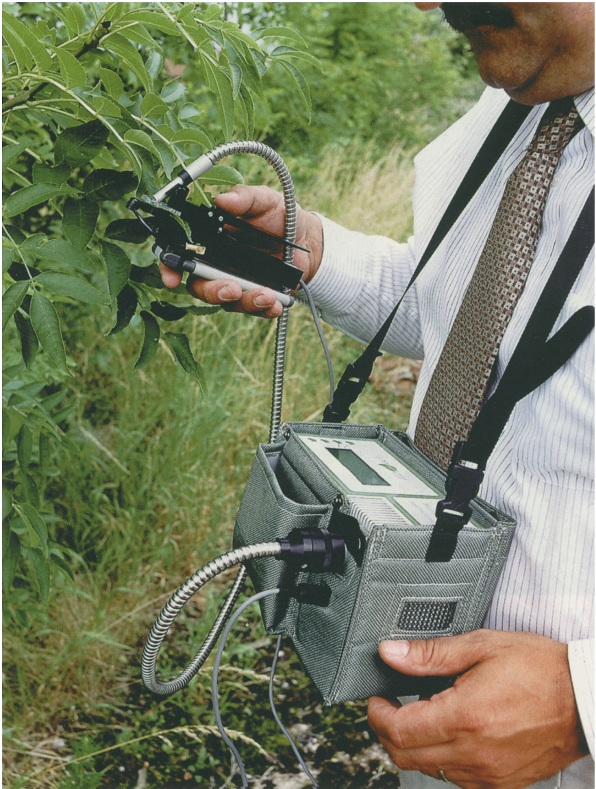
XI Measurement of photosynthesis in the field using the Hansatech FMS 2 Pulse Modulated Chlorophyll Fluorimeter. This portable fluorimeter contains all the light sources and electronics necessary for measurement of chlorophyll fluorescence during photosynthesis under natural light in field conditions. (Courtesy: Hansatech Instruments Ltd, Pentney, Norfolk, UK.)
